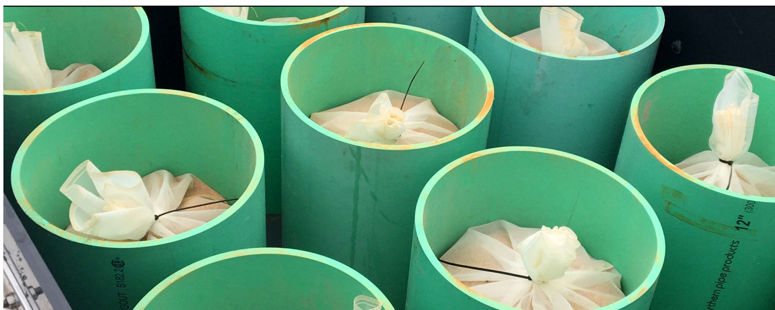
Figure 5. CAPTure™ box interior with filter vessels and filter media bags.
